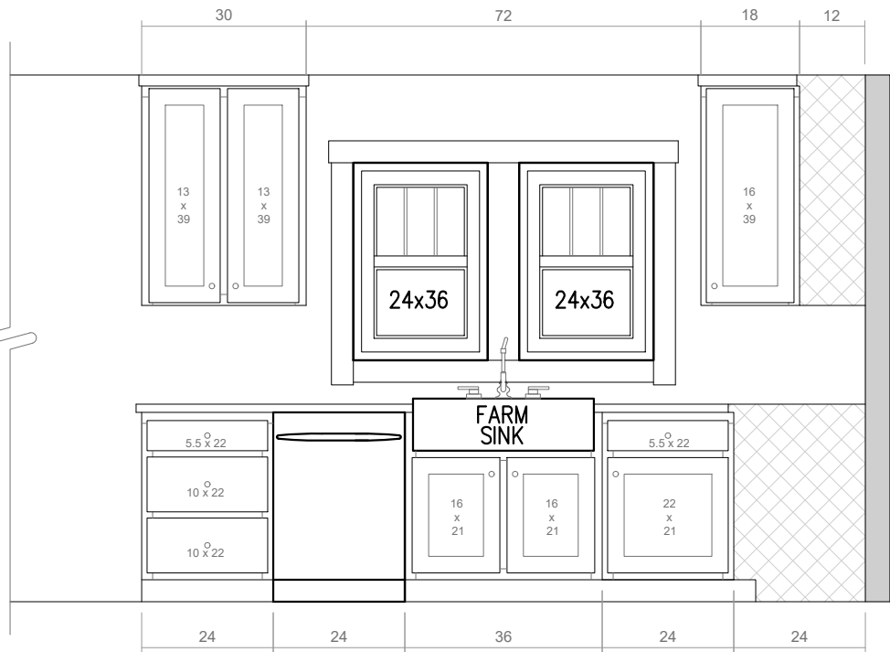
KITCHEN ELEVATION @ SINK / DISHWASHER
