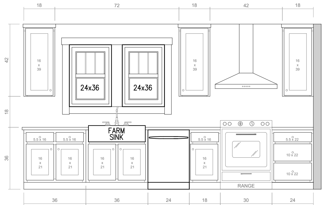
KITCHEN ELEVATION @ SINK / OVEN WALL WITH
